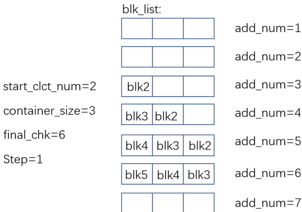
Fig 16. Illustration of the queue maintained by AutoSteper.
