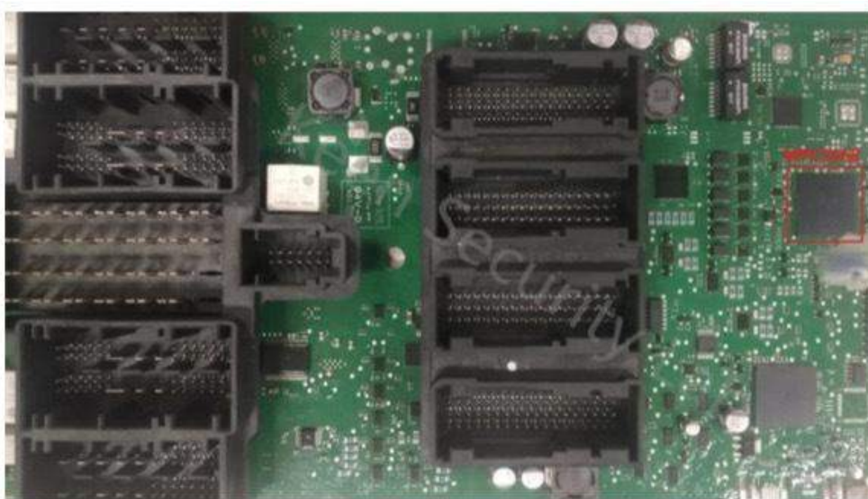
Figure: Mainboard of Central Gateway Module
