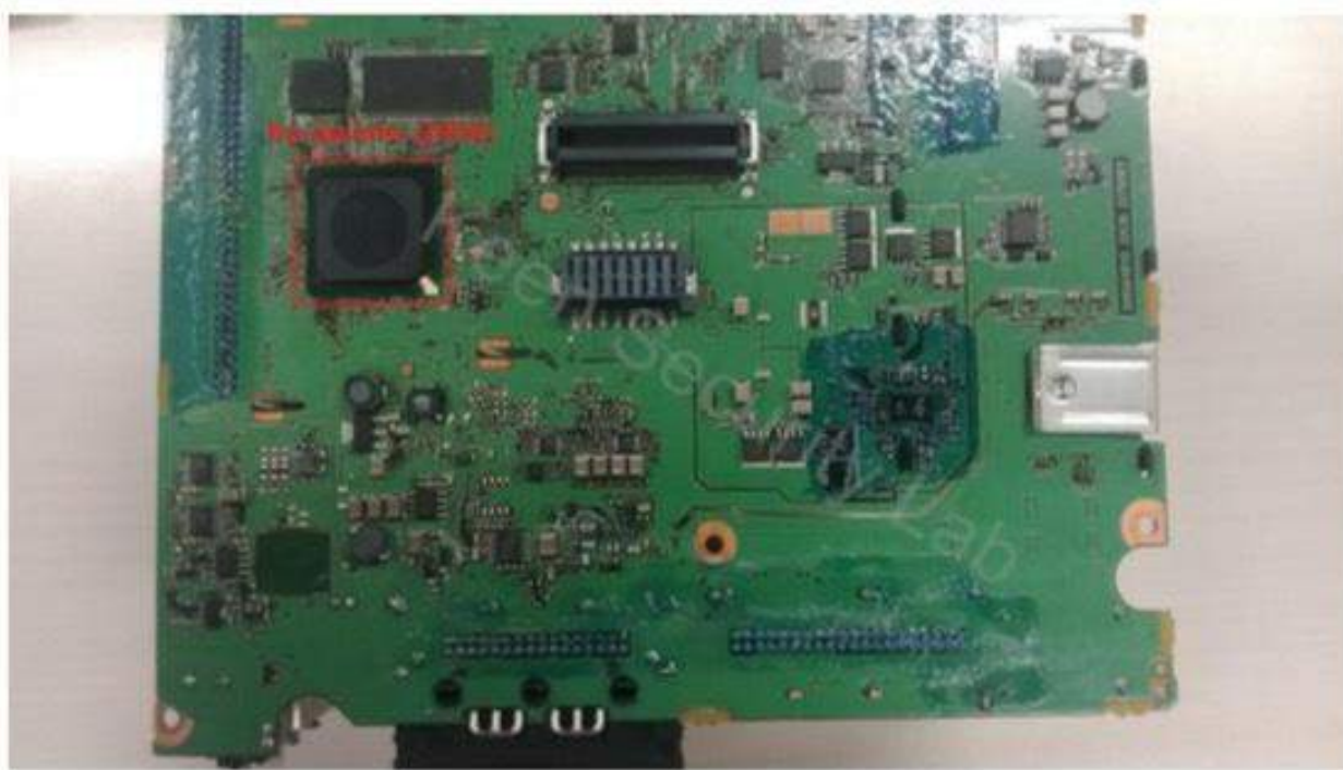
Figure: Mainboard of the Low-Layer System (hu-jacinto) in NBT
