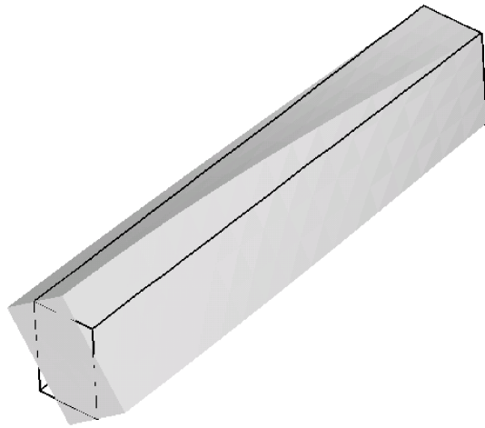
Figure 10: First torsion mode
