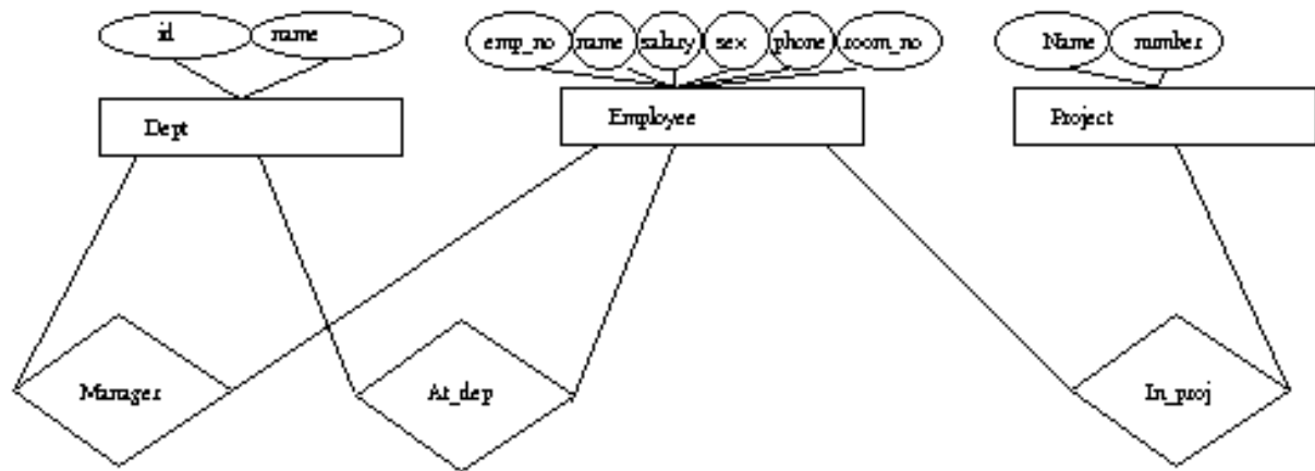
Figure 3.1: Company Entity-Relation Diagram
